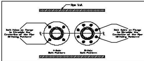
Figure 4. Flange Orientation
