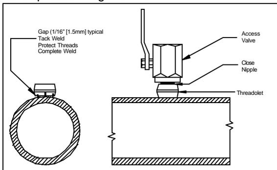
Figure 4. Weld Gap
